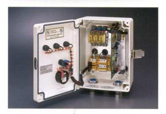
The X76AST-4X, Three-Channel Leak Detection System, is designed to give years of reliable trouble-free operation. Perfectly suited for the above ground storage tank owner, the X76AST-4X is supplied in a weather tight, corrosion proof, NEMA 4X enclosure, which is suitable for installation indoors and outdoors. The system size, 7-1/4"W x 9-1/4"H x 5"D, is easily installed even in the smallest of locations.
