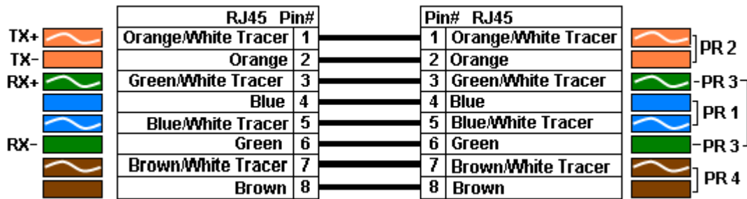
Illustration 31: Ethernet Patch Cable
