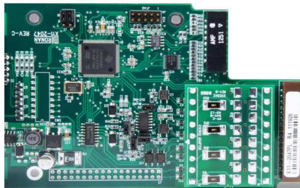
Illustration 18: Power Selection Adapter Mounted on Alarm Module
