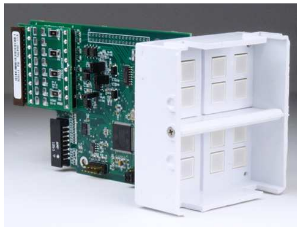
Illustration 13: Redundant Binalarm Plug-In Module
