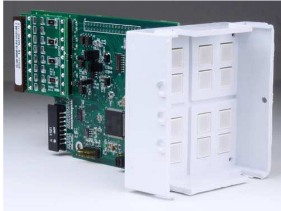
Illustration 12: Redundant Monalarm Plug-In Module
