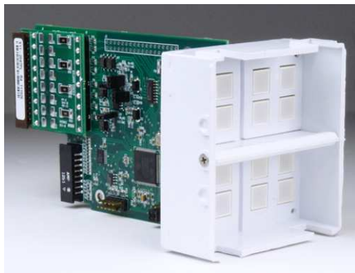
Illustration 9: Binalarm Plug-In Module
